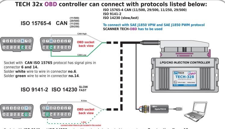
Socket with ISO 9141 and ISO 14230 protocol has signal pins located in connector no.7 and optionally no.15.
